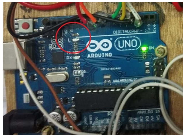
Fig 10: Device exits Configuration Mode: Yellow LED turns OFF
